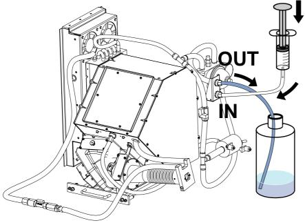
Image 2-5 Draining cooling liquid completely
